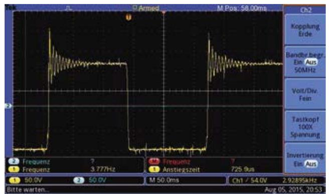
Test unit on connection A. The pressure increase is un-damped and shows the sharp pressure peak with transient response and the resulting shortened pressure dwell time. The pressure drop is un-damped and falls sharply to nearly 0 bar.
