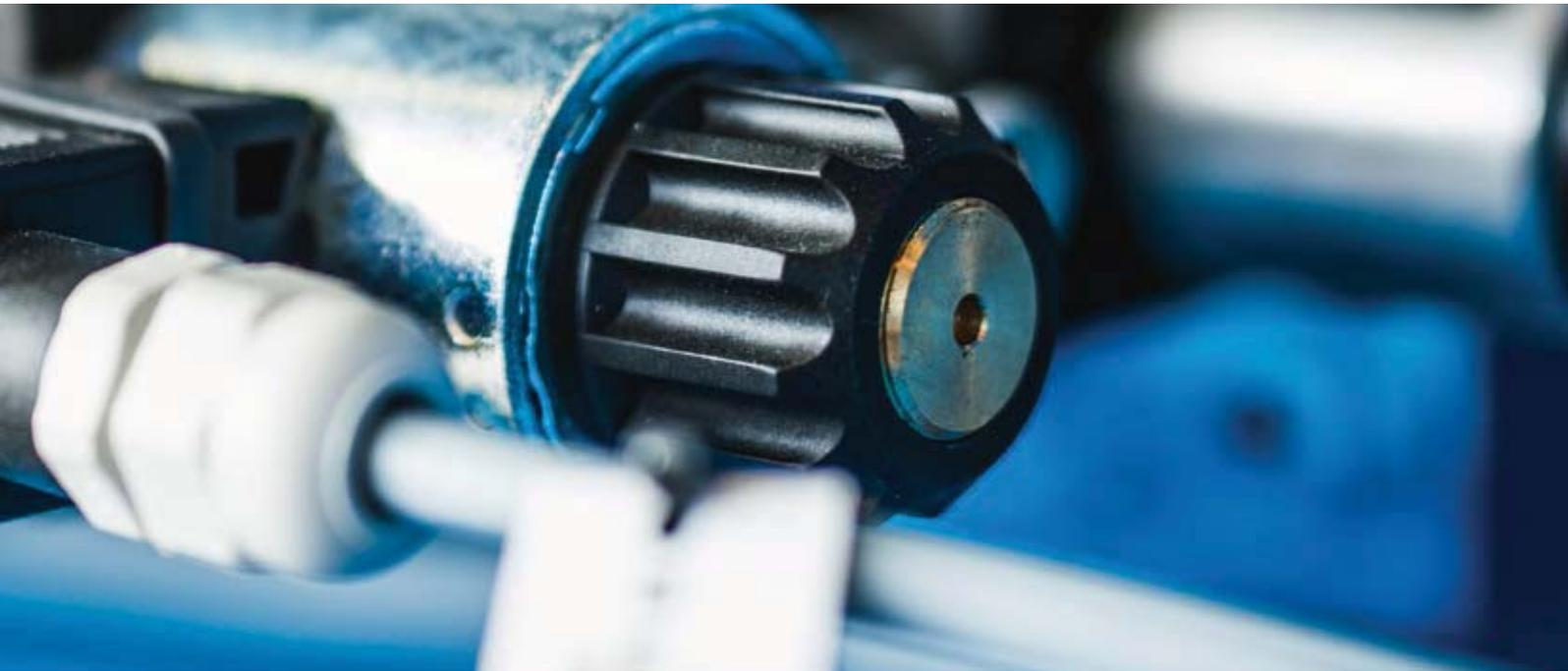
This test bench tests hydraulic pumps and motors up to 450 l/min. at a maximum pressure of 500 bar and subjects them to a performance test before they are delivered to the customer.
