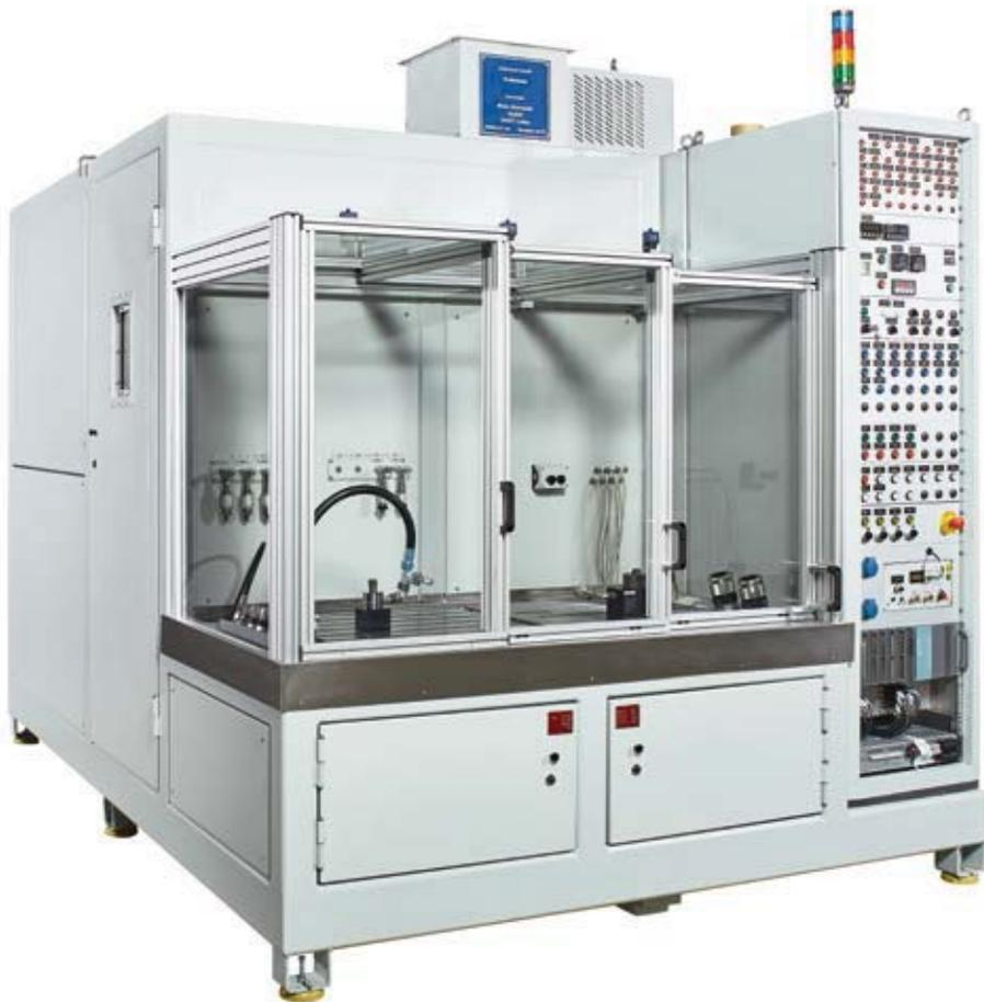
Universal hydraulic and valve tests in open and closed circuits are performed on this test bench. Maximum volume flow 150 l/min. and maximum pressure of 560 bar.
