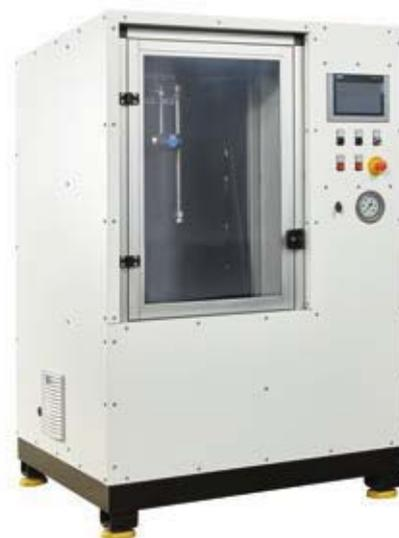
Application example of a pulsation test bench. This test bench can test the life cycle and fatigue strength of parts and components under real conditions.
