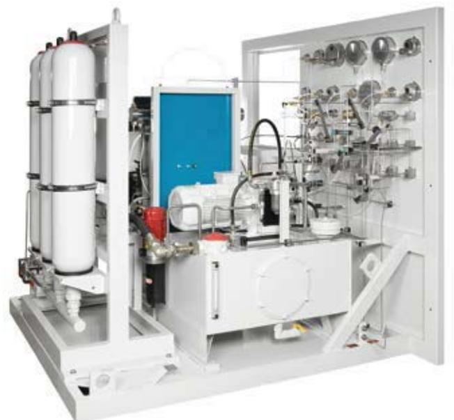
Application example of a customer-specific high-pressure test bench. This test bench tests high-pressure valves up to 5,400 bar.
